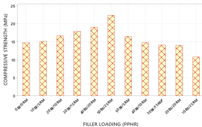
Figure 4. Effect of banana fibre and rubber modifier on the compressive strength of natural rubber vulcanizates
