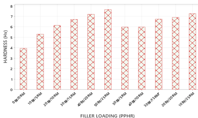
Figure 5. Effect of banana fibre and rubber modifier on the hardness of rubber vulcanizates
